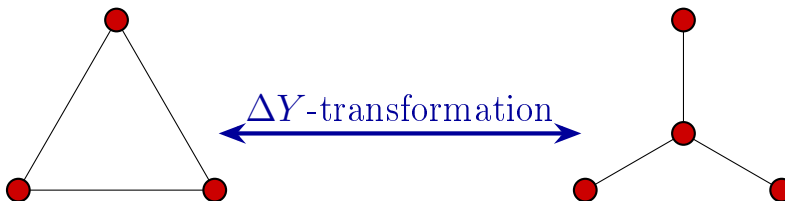
Figure 1.18: The \Delta Y -transformation.
